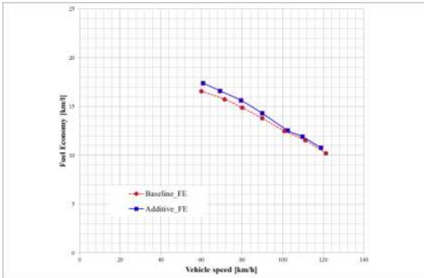
**CVS 75 Mode (equivalent to FTP 75 Mode)**
