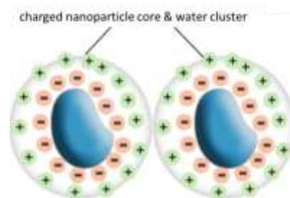
Due to the coulomb repulsion, the charged cluster does not agglomerate and stay as fine mist form and mixes with air uniformly in the combustion chamber. The electrostatic binding within the cluster prevents water from entrapping the fuel.
